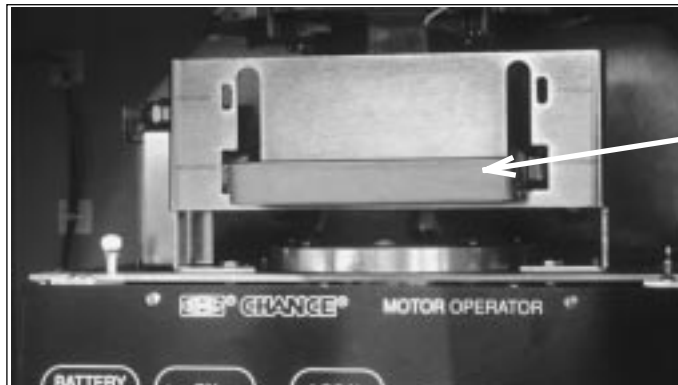
Photo A Shift handle in DECOUPLED position
